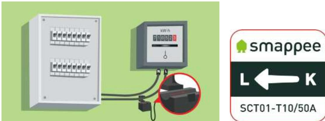
3. Place the current clamp over the L cable. Make sure that you properly close the clamp by pressing your thumb on the side until you hear a click.
