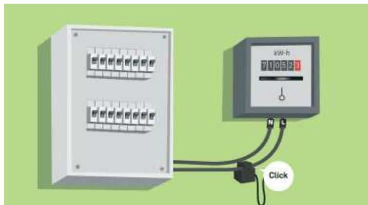
4. Plug the end of the clamp cable into input 1 of the Smappee monitor.
