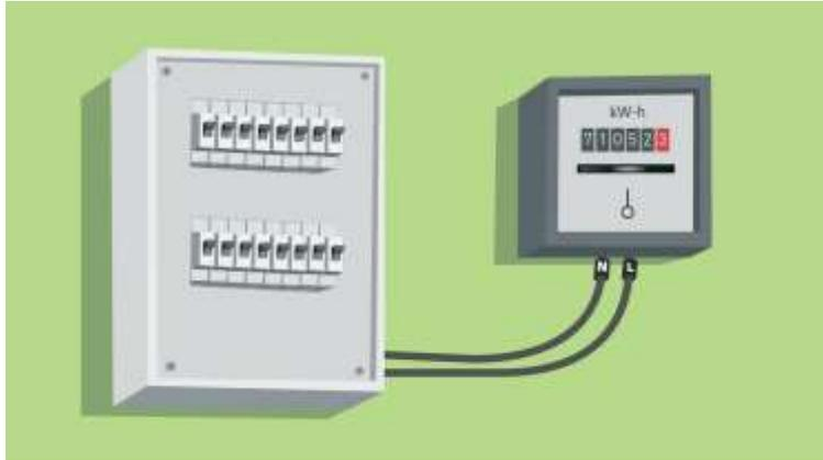
2. Then take the current clamp and check for the symbol **L ← K** in the clamp. Make sure that the arrow points in the direction of the normal current flow, from the meter to the fuse box. (**K** being closer to the meter and **L** closer to the fuse box)
