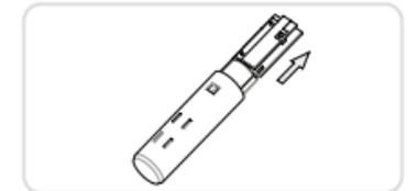
3. Remove the clear battery insulator by pulling it away from the Main Sensor.
